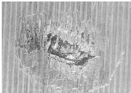
Surface fatigue on ball bearing
